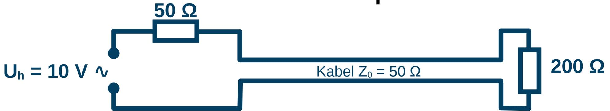
$$\begin{aligned}U_r &= r U_h = (Z - Z_0) / (Z + Z_0) U_h \\ &= (200 - 50) / (200 + 50) U_h \\ &= 150 / 250 U_h = 6\text{ V}\end{aligned}$$
